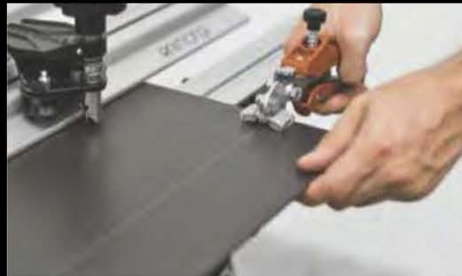
2. Cutting of Tile
