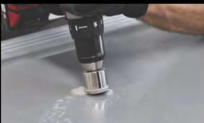
1 Round Cut with Diamond Blade Drill
